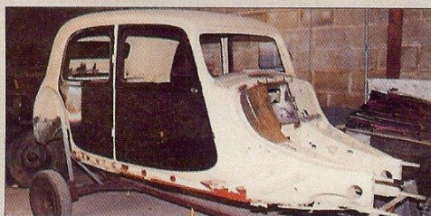
This is a rusty pre-war body shell being brought back to life at Traction Renaissance Services. The shell tapers sharply at the front, narrowing to the four mounting points for the front suspension cradle/crossmember.
