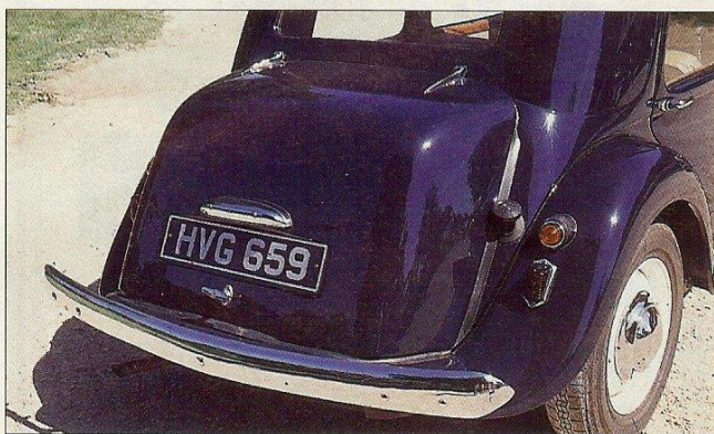
Right: The 'hump back' bootlid on post 1952 cars hides the spare wheel.
