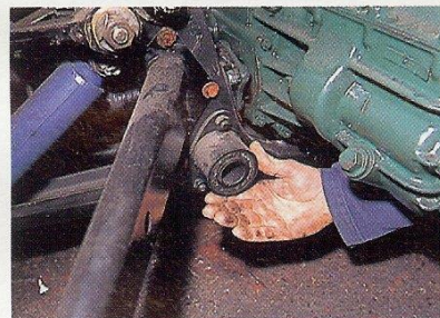
Front suspension bushes weaken with age and oil contamination, and replacement is a major operation.
