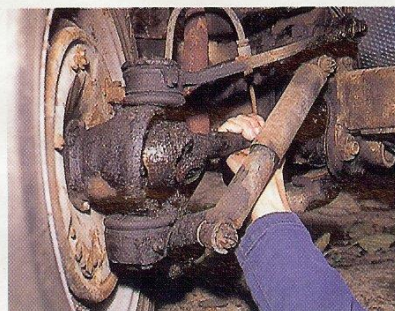
Rock driveshafts to see if there is play in the CV joints; complete shaft replacement is the best bet these days.
