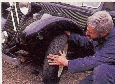
Look for tell-tale wear on the inside edge of tyres. It spells front suspension trouble and can become severe.
