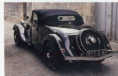
Hood panel unzips so all passengers can communicate
