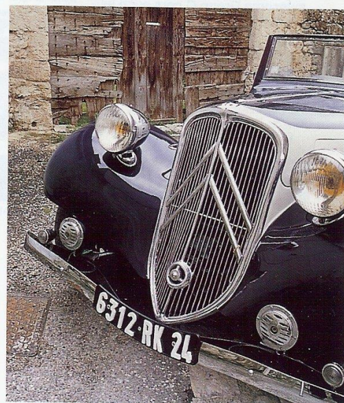
This Traction has external rather than concealed horns
