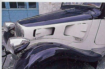
From 7B-on, front-most bonnet vent opened forwards
