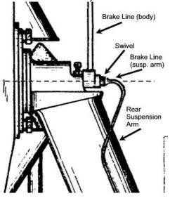
in Oldebroek, the Netherlands- offer conversion kits that do the job, but as always quite a bit of tailoring is needed to make everything fit nicely. The drawings show the original lay-out of the system and the picture demonstrates what it looks like after the modification. It included bending and flaring new brake lines, both on the fixed part of the car and on the rear suspension arms. But... it works! I still find the flexible brake lines a bit too long, but that is merely cosmetic.
