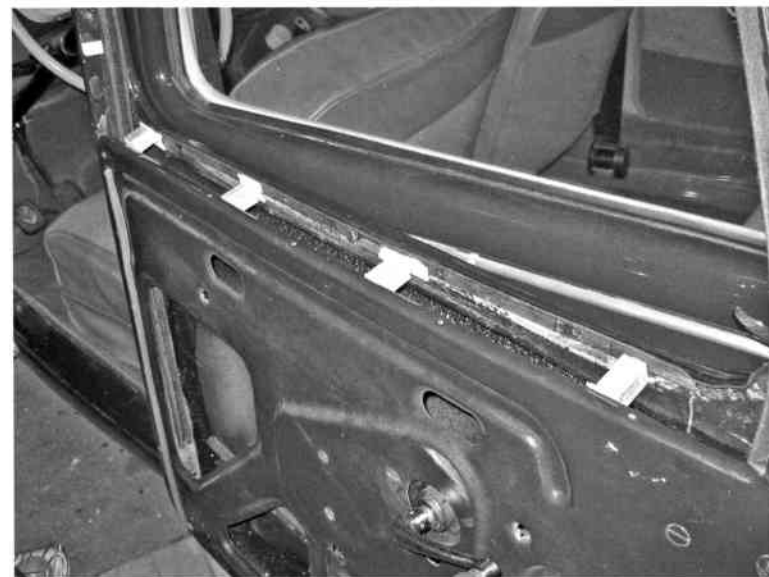
Photo graph 8 - fixing the skim rubber in place
