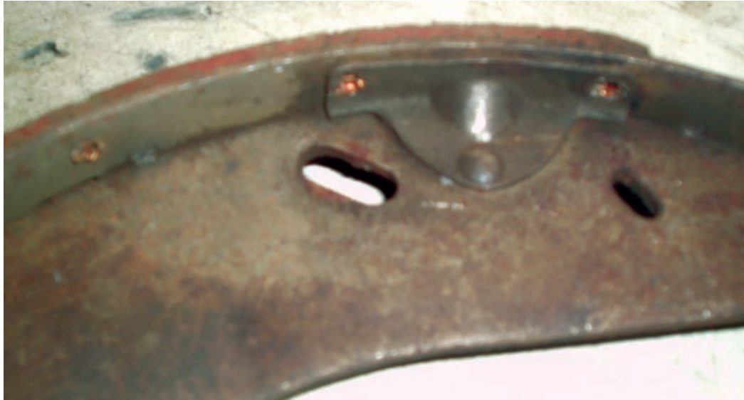
Photograph 2 reinforcing bracket of trailing brake shoe showing incorrect relining with rivets through reinforcing bracket.
