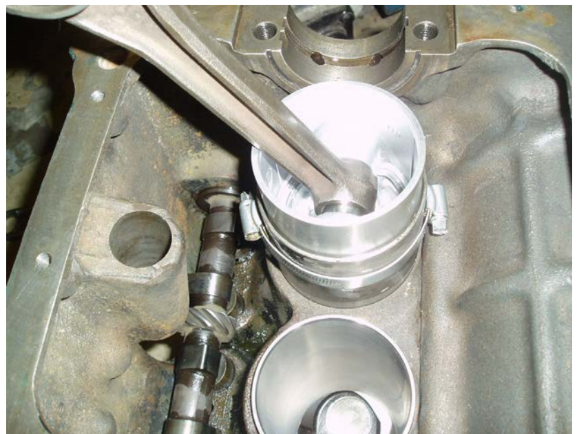
Top : photograph 1 - inserting the piston into the home made piston ring compressor Bottom : photograph 2 - fitting a piston using the piston ring compressor
