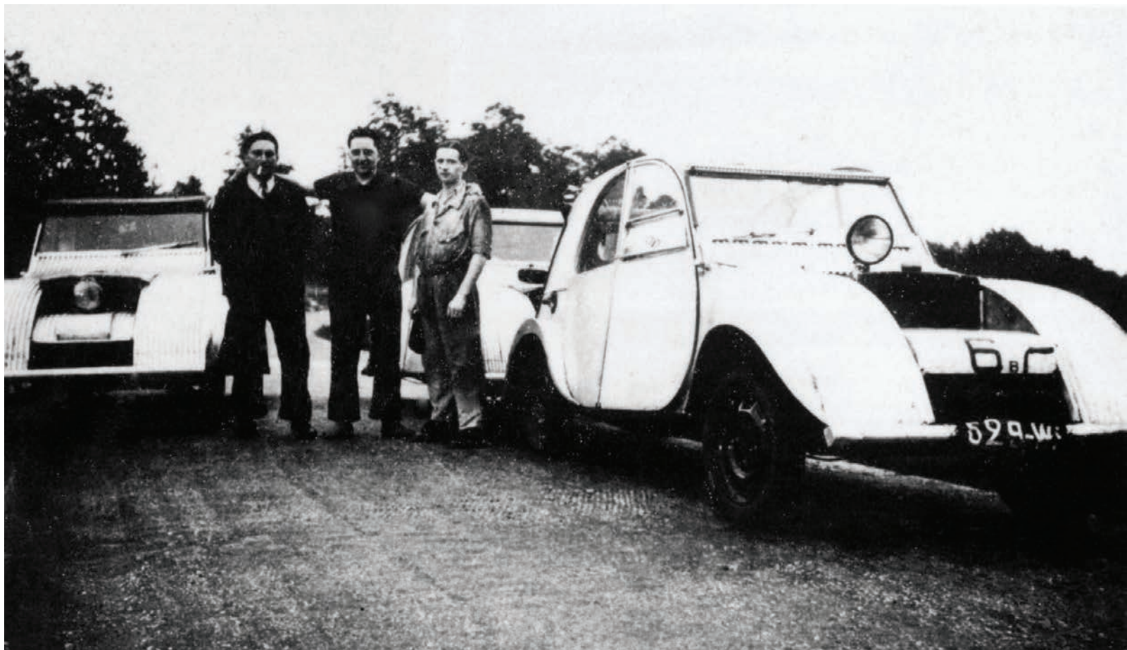
Bottom : La Fertr-Vidane 1938. The only existing photo of the prototype 2CVs. The right-hand car is the air-cooled twin, the other two are water-cooled fours .
