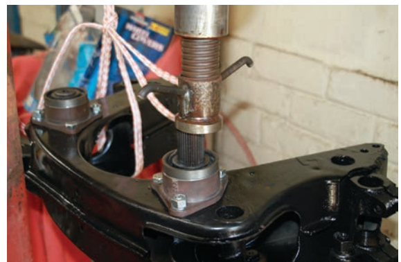
Top - fitting the silent blocs Bottom - reassembled as new
