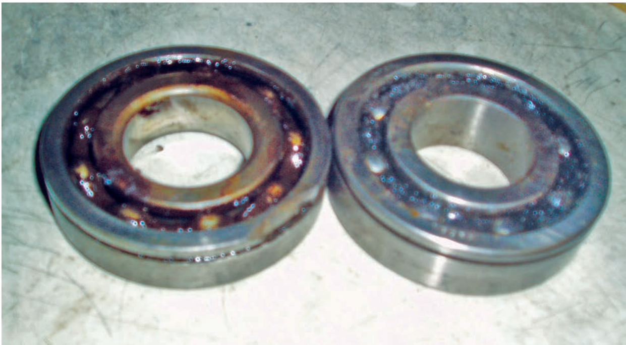
photograph 1 - pre 1950 (left) and post 1950 (right) outer front wheel bearing
