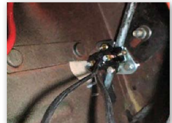
AES switch fitted to selector rod under dash
