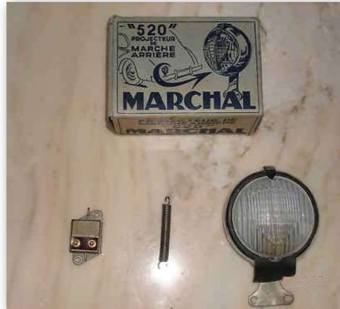
Marchal 520 reversing light, switch and spring
