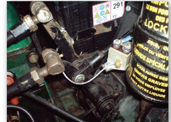
Spring replaced with cable
