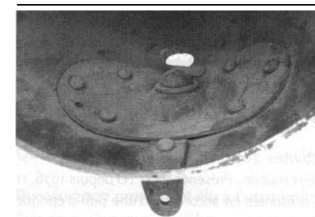
Centre fastening on shell for retaining screw of Marchal rim - pre war 15 mm - post war 6 mm under the shell
