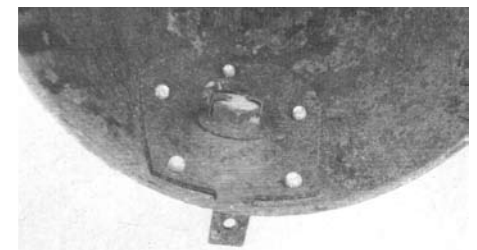
Rim retaining bracket on Cibié shell
