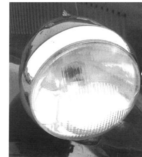
Cibié ABTP 500 from June 1955 (with new reflector having the hole for the bulb holder reduced to 42 mms in diameter)
