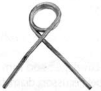
Cibié fixing spring that holds reflector and lens to rim
