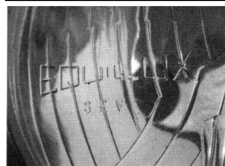
Equilux detail on Marchal ABTP 435 and 478 lenses
