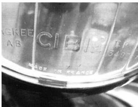
Cibié flat glass telltale in the form of rhombus known as "diamond point" (years 1936-1939).
