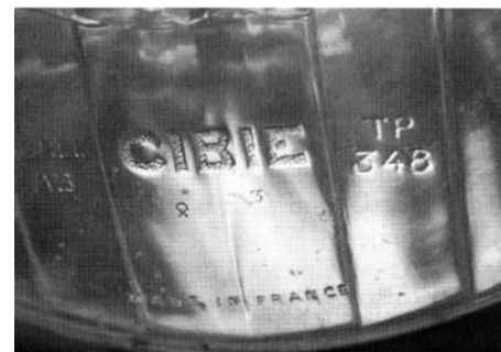
Cibié glass "cockscomb" telltale with rhombus base (1939-1941) Telltale ref. 2600A shown in the catalogue extract on the next page.
