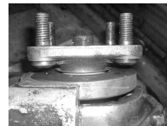
Coupling and oil seal in gearbox. The collar is not interfering in any way
