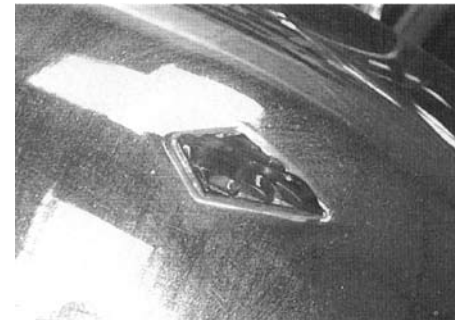
Cibié glass "cockscomb" telltale with rhombus base (1939-1941) Telltale ref. 2600A shown in the catalogue extract on the next page.
