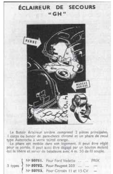
The Autoche GH with integrated reversing light. Dismounted it is used as portable lamp
