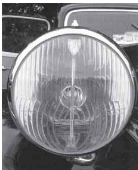
New light units appeared in 1951 on the Equilux headlight (Equilux ABTP 436A and 436 lenses)
