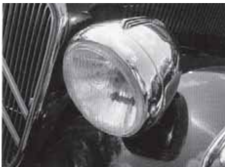
Marchal European Code optic fitted to a 220 mm shell using the crown adaptor
