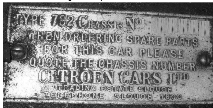
A Slough VIN plate that has been removed and re-fixed with screws
