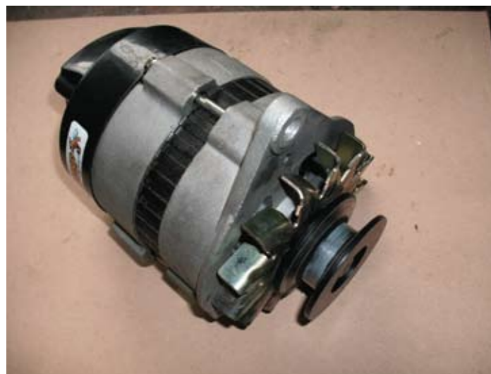
Modified Pulley in Place
