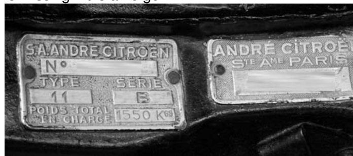
On the left a French VIN plate, on the right the French coque plate, showing how the plates should be fixed.
