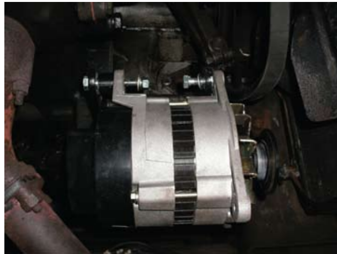
Photograph 5 (above) shows the alternator mounted on the brackets but swung down to show the spacers and bolts (not tightened!).
