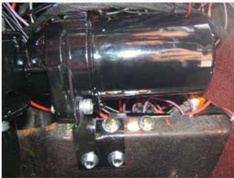
Photo EZ power-2 The power unit installed, showing the modified fixing bracket and draw-up plate (behind the up-turn).
