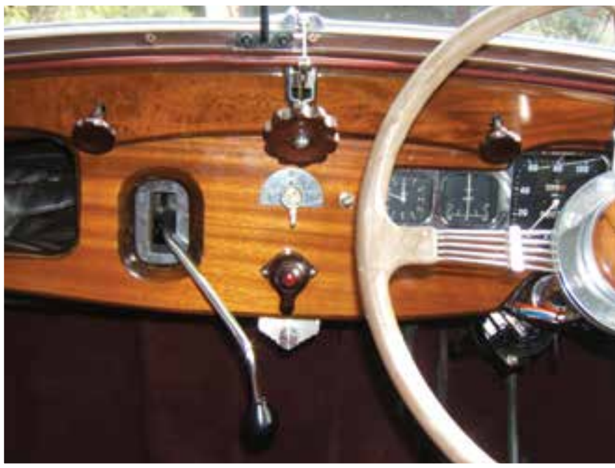
Photo EZ power-1 The only noticeable give-away that the car has a powersteering unit installed, is the small controller dial and knob under the indicator switch.
