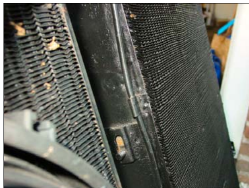
Left radiator is original. Note larger cooling block on refurbished radiator (right).
