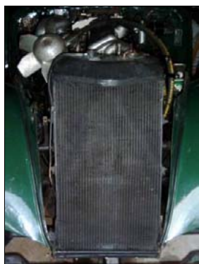
15-Six radiator with no crank hole
