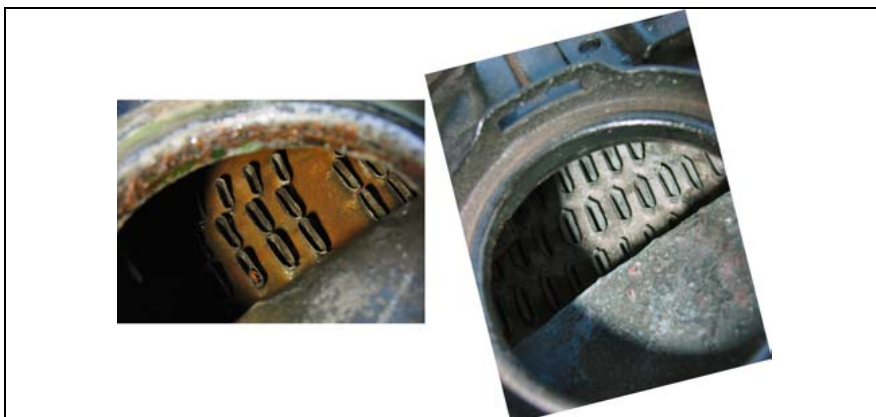
Left image shows original cooling block with pipes partly covering each other and close together. Right image shows cooling pipes in new cooling block. Note the even partition across surface and increased space around the pipes.
