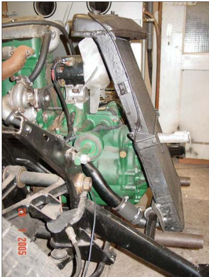
General configuration of 15-Six radiator. Tunnel around fan and side brackets have been removed for better view.
