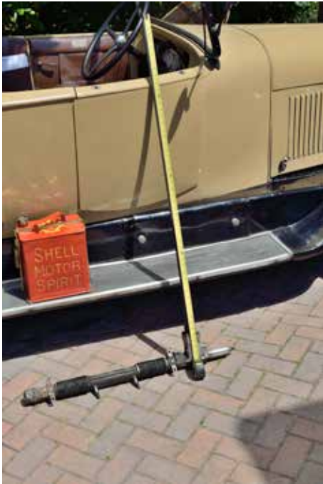
Left The steering column - surprisingly, there is a lot of it - it is about 58" long
