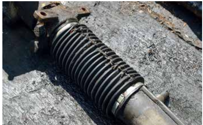
Right. Way back in the distant past, someone (the tea boy perhaps) was sent under our car to sew new gaiters onto the rack. Can you imagine?
