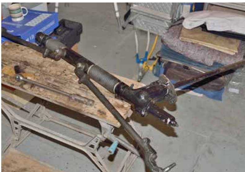
Reconditioned rack from the club with drop arms in place.
