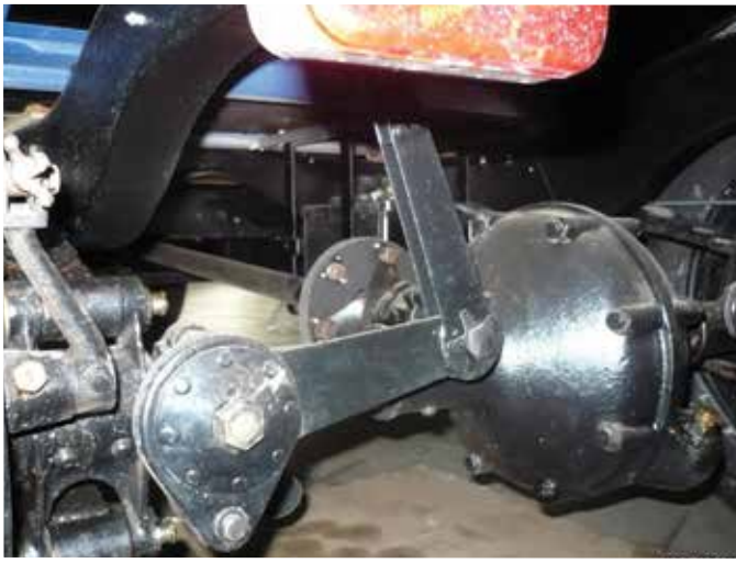
Above - the rear axle of a Citroen B12. The shock absorber has been bolted to the rear axle casing. A large stud locates and prevents the outer shells of the Hartford style shock absorber from rotating. A pressed steel arrow (at about 2 o'clock) is intended to assist the mechanic in achieving equal rates of damping on the axle
