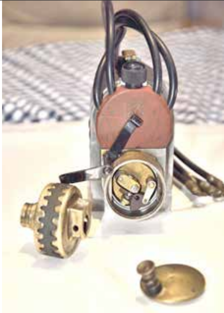
Above. End view of a Rousseau Bignon magneto showing the numbered HT leads, points, two cams and the cover plate. The points rotate, the cams stay put. From the cover plate is taken a lead which is used to earth the low tension circuit within the magneto and thereby stop the engine.
