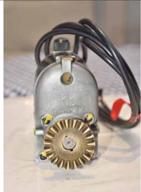
Front view of the RB Type 10/4. Behind the toothed flange and not visible is an arrow that shows magneto operation to be clockwise. The little window at the top is to facilitate initial timing of the unit to TDC on No 1 cylinder.
