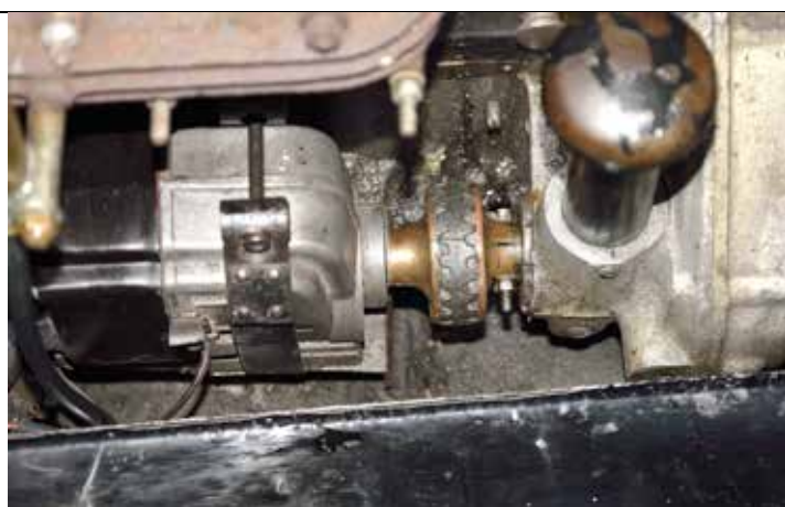
Above right, an almost identical Citroën engine, but this time with the Simms Vernier Coupling.
