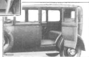
Diagram showing the Brougham in use as a light van. The rear seat and squab are removed and the platform is inserted.
