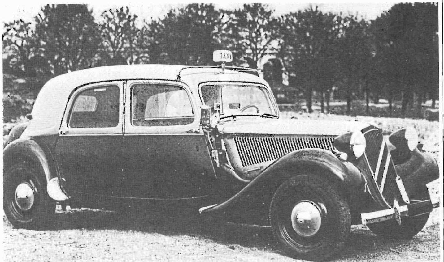
The first Familiare taxis were launched in 1935, without any great success. This example is fitted with a sun-roof, semaphore indicators, and a windscreen modified to take the meter. Note the full rear doors, twin air flaps and the flat headlights. Pick up charge was 1.25F.
