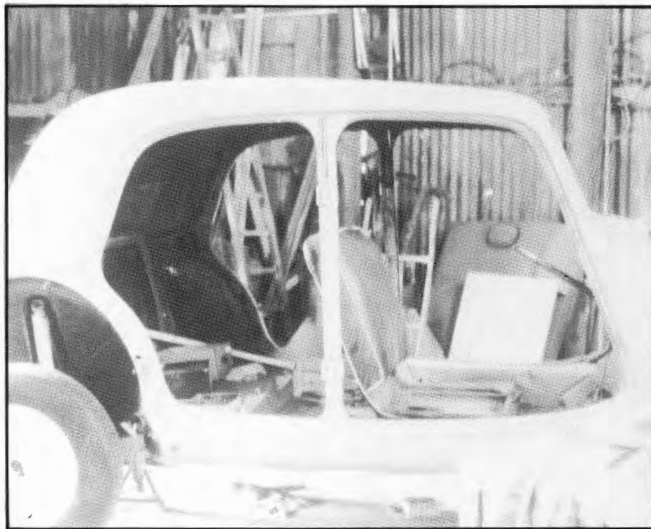
Bodywork prepared and ready for paint shop.
