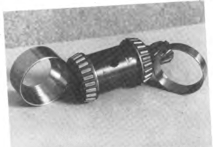
Pinion ready to accept steering column and be fitted to steering box.
