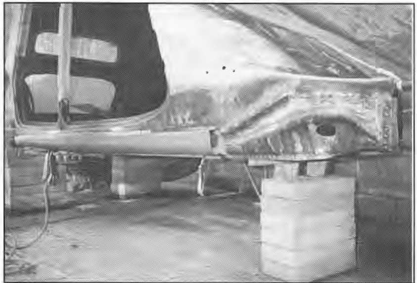
Outer sill screwed in place ready for plug welding
