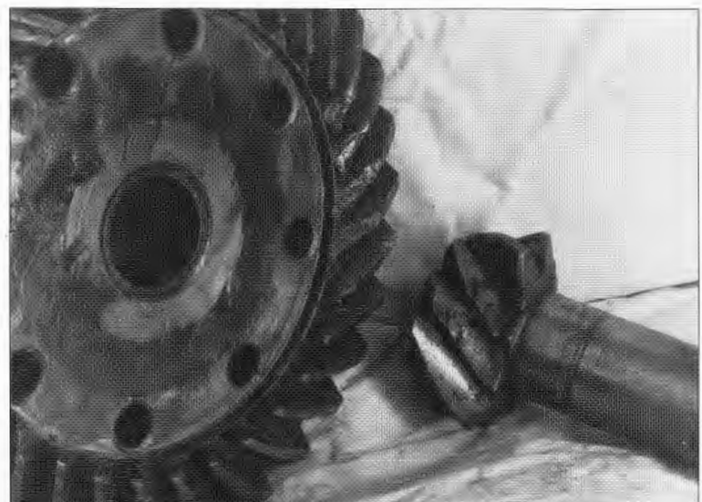
Typical damage to crown wheel and pinion
