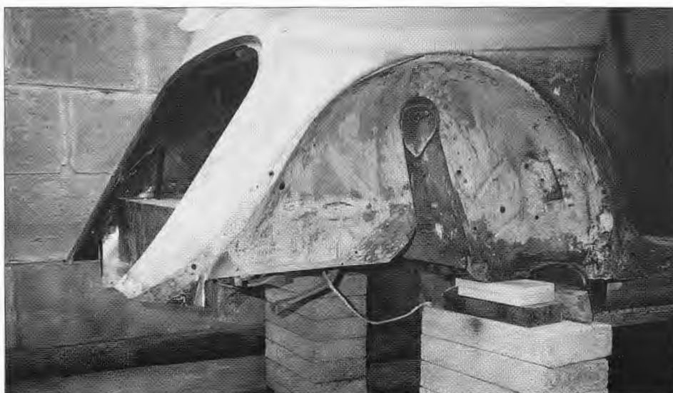
As with the left side, before removing the rusted portion of right inner wing, detailed measurements were taken and a replacement panel was made. I found on this Slough 6 that the right-hand inner wing was actually a different size to the left-hand one!
