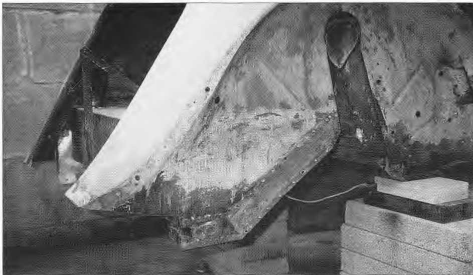
New section for rear inner wing and boot floor, the inner wing section was put in place first, followed by the boot floor. The boot lid was used as a template to keep the boot aperture correct.
