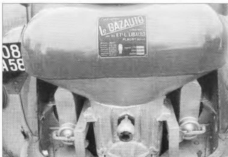
The generator and its firebox. Louis Libault, who succeeded in markedly reducing the weight and bulk of the gazogene through co-operation with the competition, didn't neglect to offer his patents in France and abroad for the consideration of other motorists.
