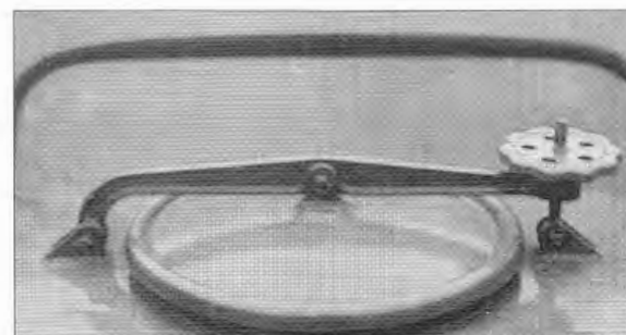
The pressure vessel cover with its locking wheel.
