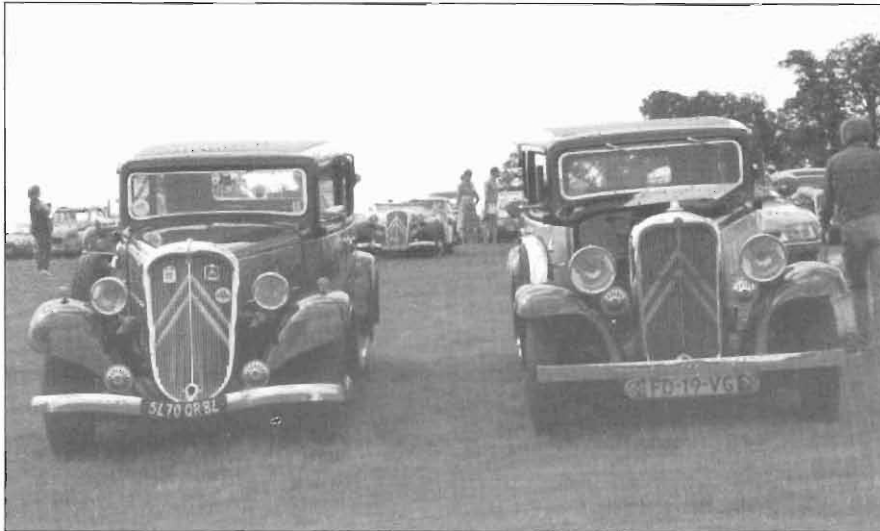
The car on the left is the Nouvel Habillage model. Note the Traction-like grille, wings, headlamps and bumper.
