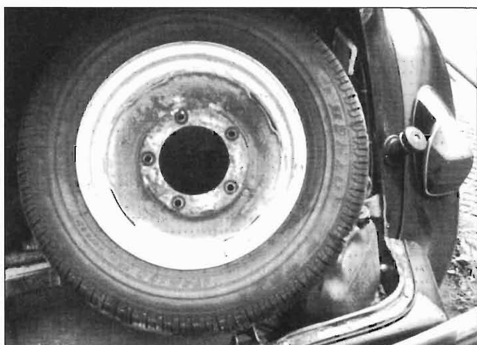
16" taxi wheel rim, welded to Light Fifteen wheel centre. Both items originally manufactured by Rubery Owen
