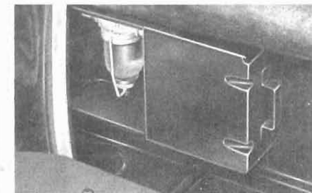
The petrol filter in the rear boot (fitted only on early series)
