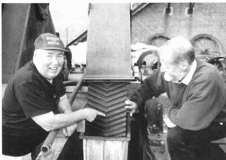
Rally organiser Barrie "Brick" and TOC Chairman Alec Bilney inspect a double helical gear which was part of the winding mechanism - they didn't find a makers' plate.
