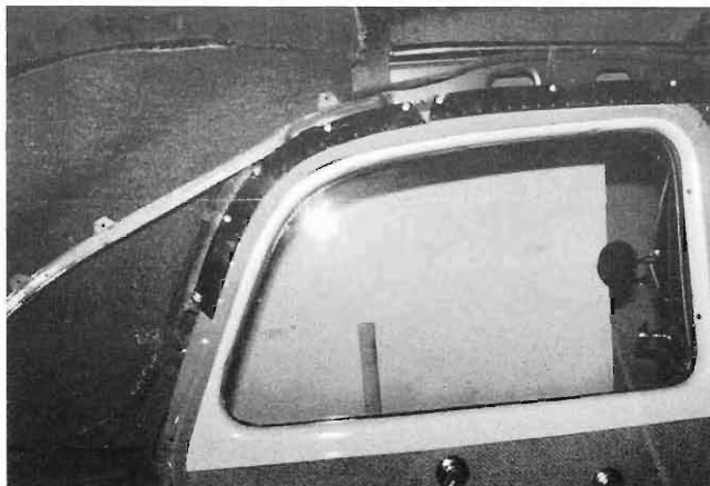
Pic 7 - The flexible side-plates, with triangular teeth which grip the edges of the stretched head-liner.
