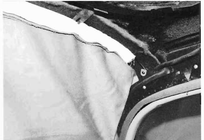
Pic 10 - The stretcher-bars are screwed to the lugs at each end; the fabric pockets are pierced and held by triangular metal hooks in the roof.
