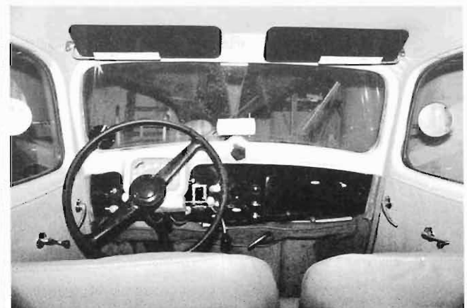
Pic 12 - A single hinge piece modified to mount twin sun-visors.
