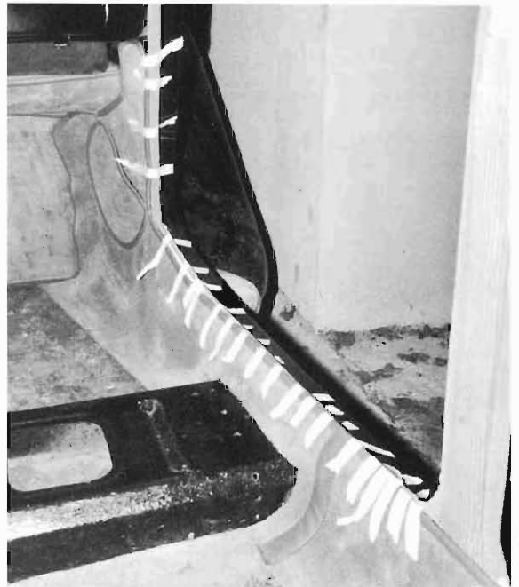
Pic 15 - Masking-tape holds the carpet liner in place while the adhesive dries.
