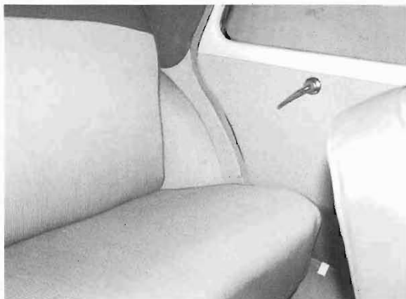
Pic 13 - Make sure that the upholstery material are aligned.
