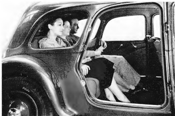
Citroën image of a 1938 model-year 11B limousine - there are Pilot wheels and the standard saloon doors used from October 1937. Note also the comet-pattern door trims and the separate Tubauto front seats. This is a delightful photo that had to be discarded from the book because of a lack of space
