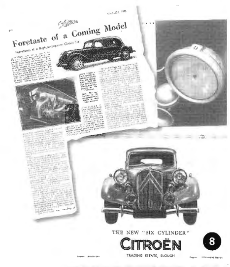
Photo 8: Comments (in the article from 1939): - (above) Citroën's f.w.d. system allows an extremely low, yet roomy, body. Note the new Michelin-wheels, now very popular on the continent. - (left) the carburetor of the six-cylinder o.h.v. engine is carefully screened
