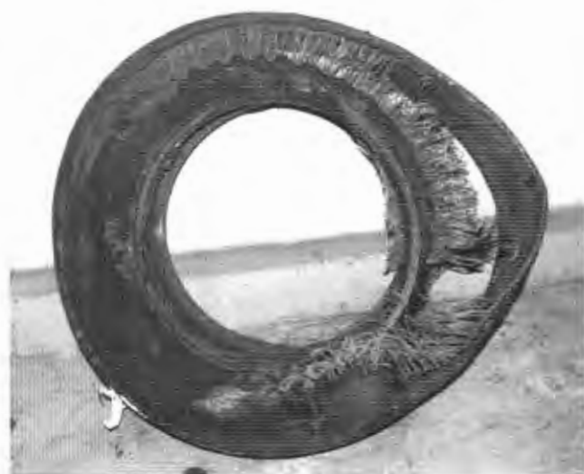
Photos from Rex Grogan's files of tyres from crashed vehicles: top - detached tread section, centre and bottom - sidewall failures in radial tyres
