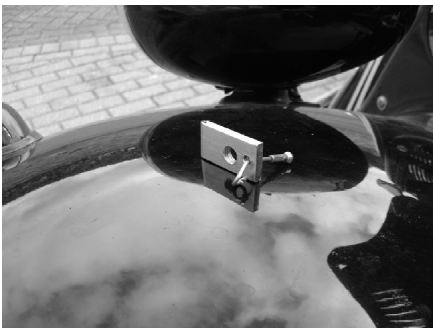
Photo 4 - one of the lock plates with it's clever little holding wire
