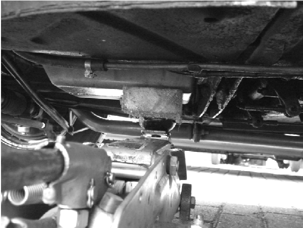
Photo 2 - Engine supported by trolley jack and wood
