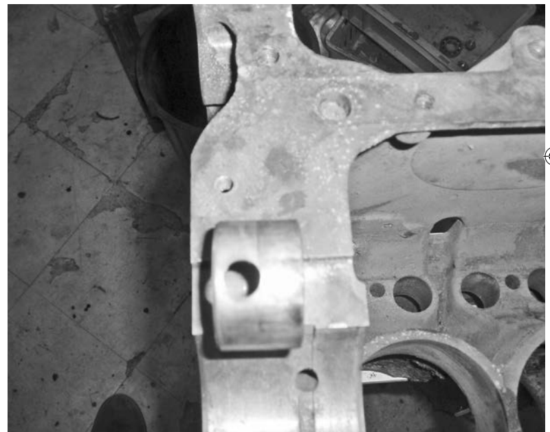
Photograph 1 - Camshaft front bush, turned to offset oil feed hole to the front
