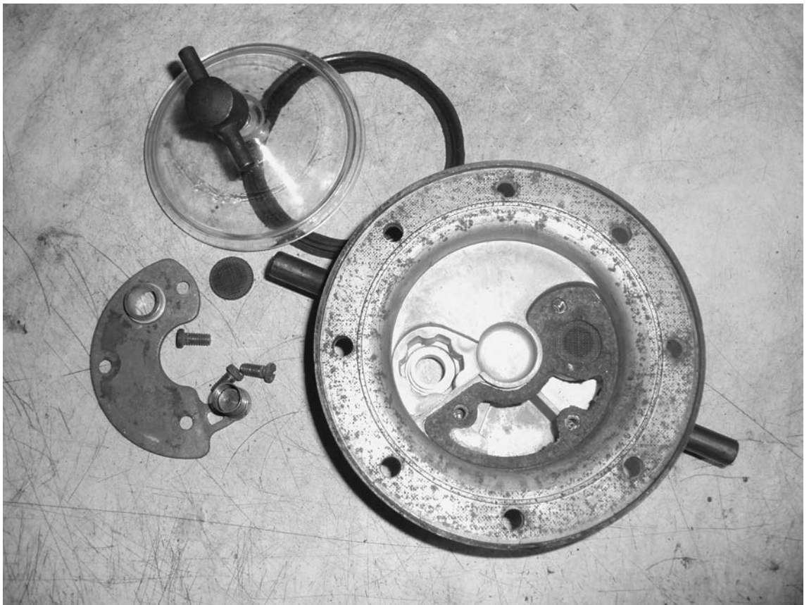
Top - stage 1 : replacing the diaphragm. Bottom - stage 2 : underneath the top part of the pump is a plate screwed to it that retains the two disc valves and their springs. Ensure the discs, springs and seatings are clean and in good order.
