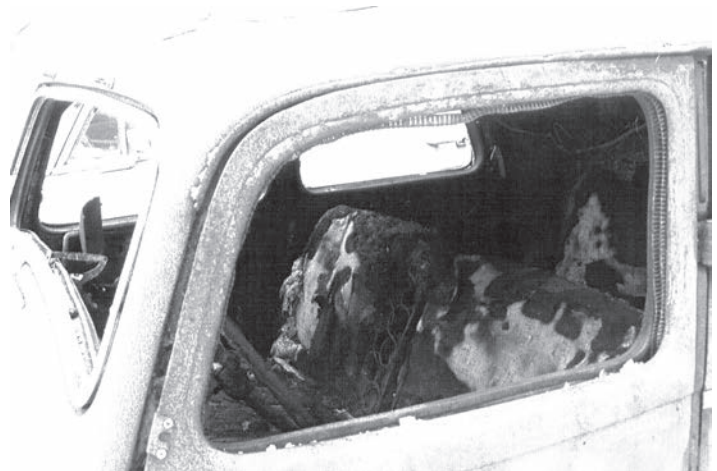
Above - cautionary tale 2 : the results of not having fused electrical circuits
