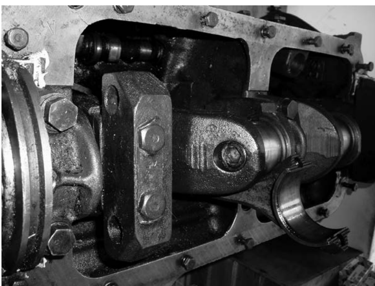
Left - cautionary tale 2 : the results of trying to bump-start a Traction Right - the correct way to fit the connecting rods into an ID19 engine
