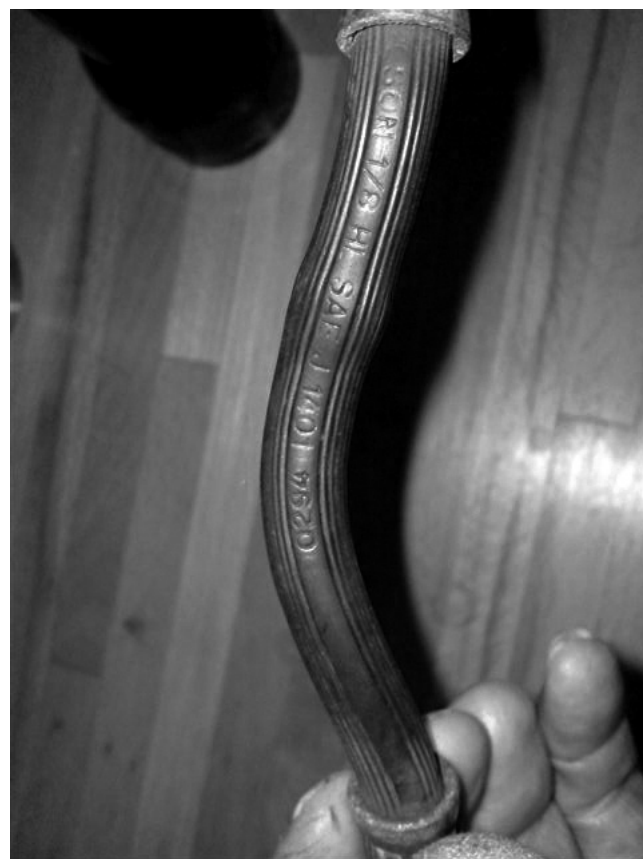
Left - Den Hewitt's perished brake hose clearly showing the bulge in the hose wall Right - the date of manufacture of the hose - 0294 - can be clearly seen in the wall
