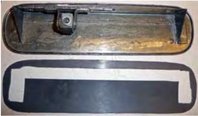
Rubber gasket glued to the inside of the cover © KBtW
