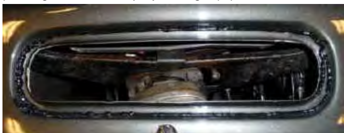
Sikaflex 291 applied to slot
