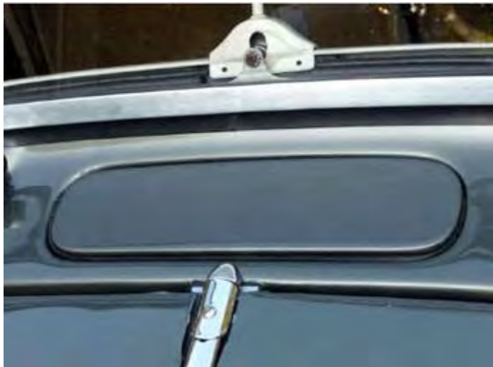
Air vent closed and watertight!
