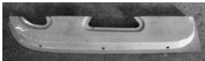
Rear door inner bottom repair piece
