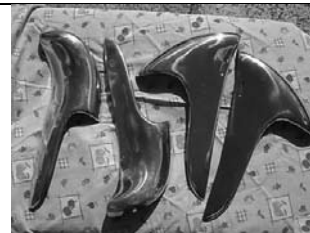
On the left a pair Sabots d’ailes 224s for the front of rear wings and on the right a pair of 223s for the front wings of big boot cars
