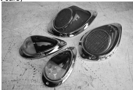
Type 229 for the front or rear indicators and type 230 for the rear stop and tail light on big boot Tractions
