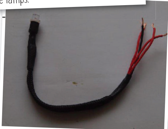
8. Completed sheathed harness.
