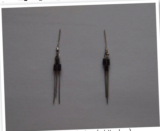
1. Common end of diodes (white bar) soldered together.
