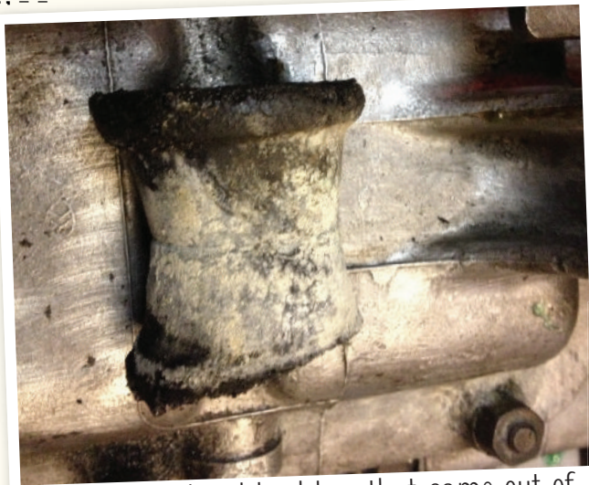
This one is the old rubber that came out of the gearbox mount...
