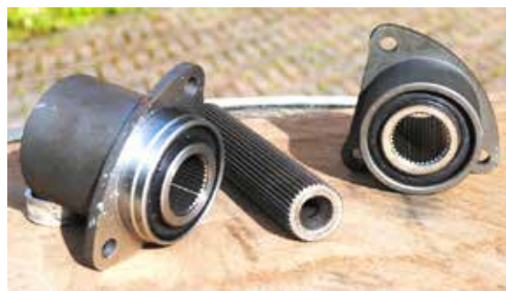
Fig 4 New silent blocs set.
