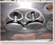
High pressure air and lots of poking restored the rocker oil supply and the machinist did an excellent job with the head.
