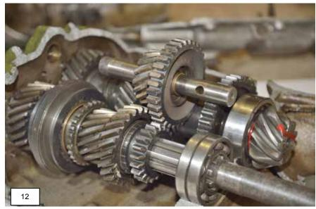
There is a tapering bronze conical shape on the inner part of the synchro (*Photo 13 & 13a*) which is a perfect match for a similar shape on the end of each gear wheel. A gentle push and they will hold together (*Photo 15*). In (*Photo 16*) are 3rd & 2nd gears on the mainshaft with a gap in between for the synchro.
