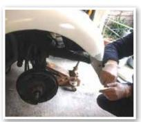
undid the castellated nut on the driveshaft. This came off suspiciously easily, and as an experiment we applied the torque wrench to the recommended reading and again tried the assembly for play. It made no difference, so we loosened the nut again and got out the club extractor, the hub and brake drum assembly came off with only a modicum of gentle persuasion, and the special tool for the castellated inner
