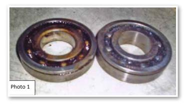
If the narrower 17mm. bearing is replaced with a 19mm. wide one it is essential to reduce the width of the spacer between the bearings ( see photograph 2) by 2mm.
