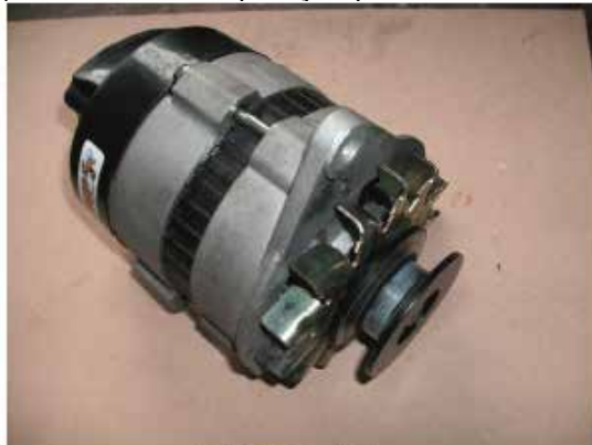
Modified Pulley in Place
