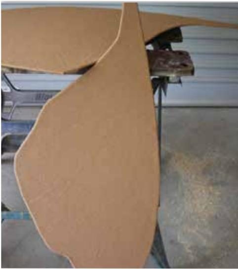
I have sewn the headlining and it is ready to go back in to the car as are the four door cards. I have also remade the two wings that fit at the back of the car interior. These use cardboard as a backing but the only one I had was warped and mouldy. Utilising 3mm ply I used the original as a pattern and covered both in the same material as the headlining.
