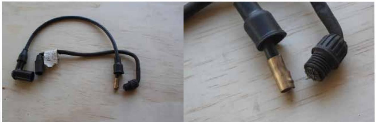
Having remade the plug leads it was time to put the new parts back in to the distributor. Either I have fat fingers or the small screws are just fiddly, but it did not take too long to put things back together. Another job I can cross off the list and the distributor can be installed in the engine.
