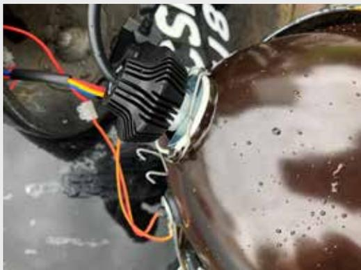
The LEDs are direct replacements for H4 bulbs but come with adaptors for P45 fittings. However, the LED's H4 flange sits sub-flush in the adaptor and the spring clip was having trouble accommodating that. I had to make up some packing pieces so that the clip held them firmly in place.
