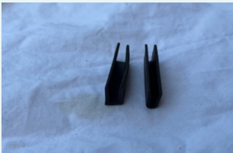
Picture 2 The internal body seam seal, 5mm wide internally (left) 3mm wide (right)
