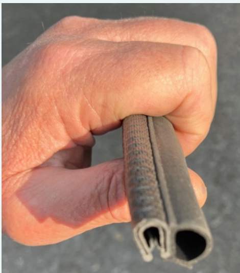
Picture 3 Alternative interior body seam seal, left side fits over body seal, right hand side is soft 'D' section
