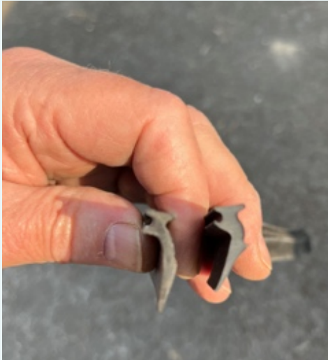
Picture 1 The old (7mm) and new (right hand) 8mm across the 'T' external windscreen 'blade' seal with the external stiffening rib
