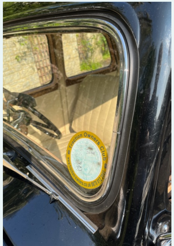
Picture 5 The external blade seal fits flush and tight to the body
