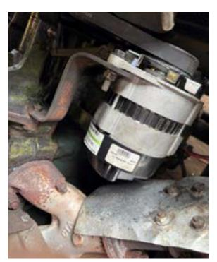
Franssen will sell you a 6V alternator kit for 380 euros or a 12 volt on for 411 euros. The kit includes the mounting bracket and the alternator is fitted with the correct pulley for the wide V-belt that the Traction uses. To be honest, I am not sure if Franssen's alternator also needs an external regulator. Pat2D offer what look like the same alternators and they do have internal regulators – but they include neither the bracket nor the pulley.
