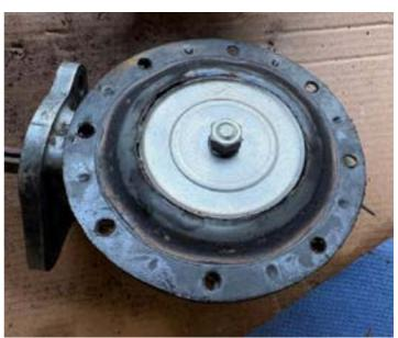
My pump is the SEV type. The top cover is metal, although some seem to be glass. Both types are held in place with a central bolt. Removing this reveals a gauze strainer which had done a sterling job or filtering out dirt over many years. This is not visible
