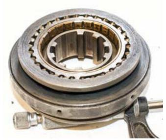
**Above left:** our 2nd gear synchro cone badly worn unlike the 3rd gear synchro cone **above right** still in good condition.
