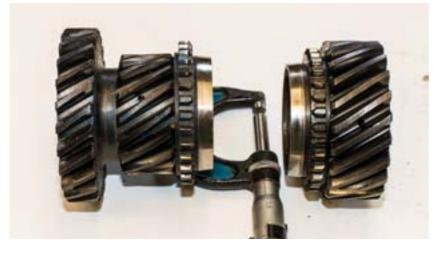
Secondly, all should become clear as I work through the synchromesh principles and failings. Left: are two gear wheels with shiny conical surfaces sitting opposite each other.
